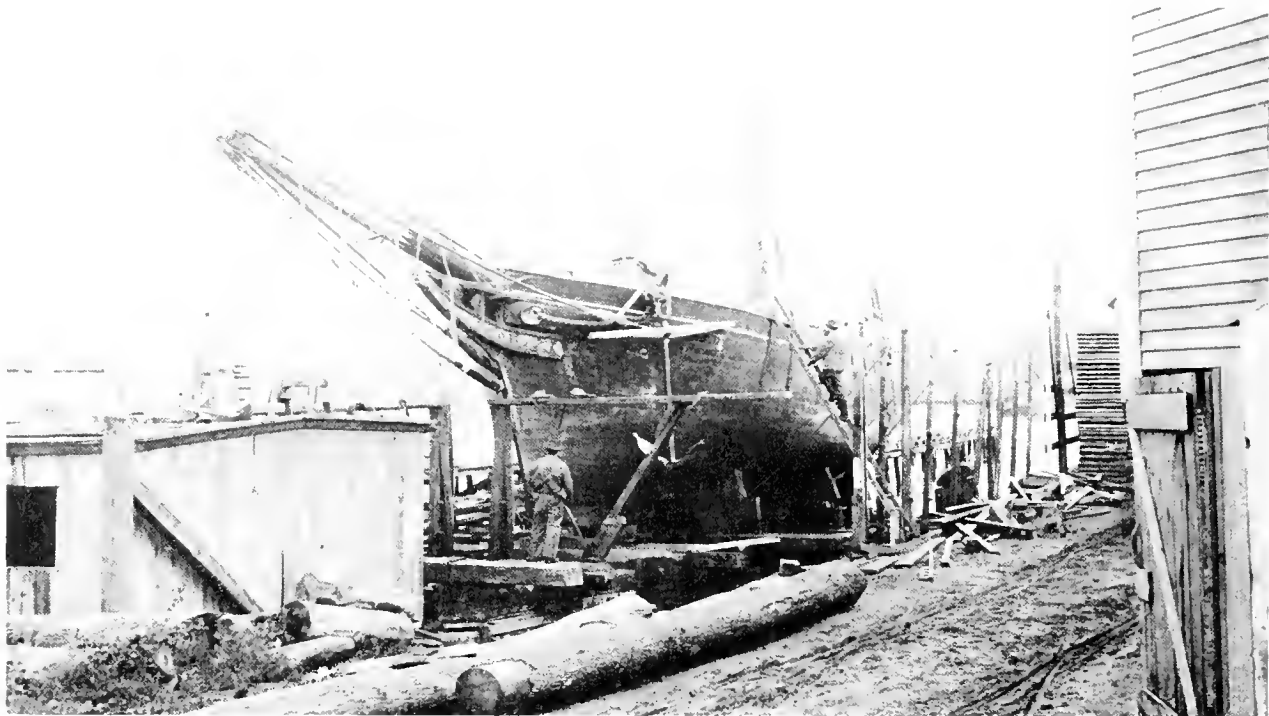
FISHING SCHOONER ON MARINE RAILWAY IN THE 1880's at Rocky Neck, Gloucester, showing the typical head work of an Essex-built fisherman of the period. ( Smithsonian photo 44791. )
